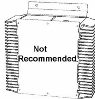
3. Ensure all heat dissipating parts are not obstructed to avoid overheating. Do not put the battery charger near any heat sources. Make sure that free space around the battery charger is sufficient to provide adequate ventilation and easy access to cable sockets.
