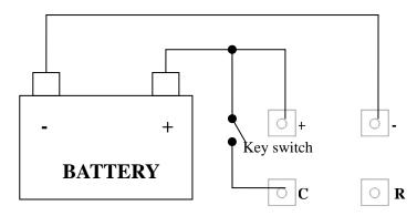
Pin R & R are relay pins, acting as switch, which can shut off the device connecting via them, when battery voltage is too low, so as to prevent battery from over discharge.
