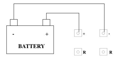
Pin R & R are relay pins, acting as switch, which can shut off the device connecting via them, when battery voltage is too low, so as to prevent battery from over discharge.
